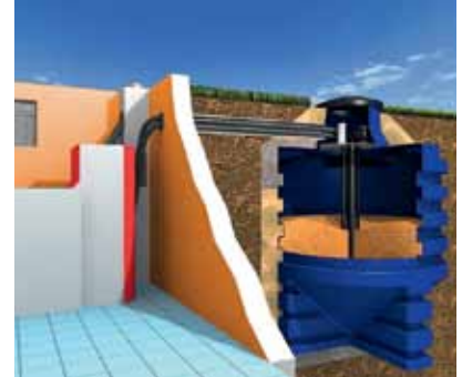
Plate 8: Below-ground silo made from synthetic materials, discharge from below
