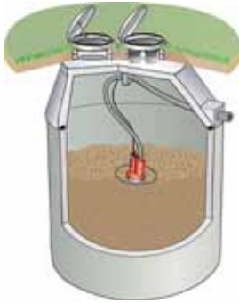
Plate 6: Below-ground silo made of concrete, discharge from above
