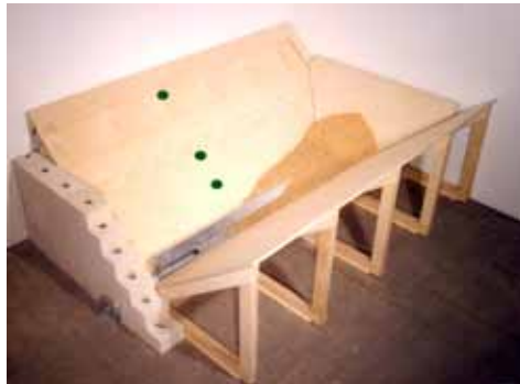
Plate 25 Pressure sensor for the filling status in an inclined bottom
